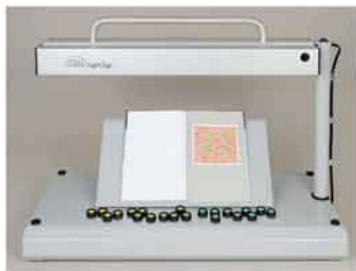
Fig. 2): Colour vision examination site “Light2go” providing D 65 standard white illuminant (Unity Color, Torso Publ., Wertheim, Germany)
